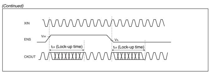
If the ENS pin is used for modulation enable control during normal operation, the set clock signal is output from the CKOUT pin at most the lock-up time " $t_{LK}$ " after the level at the ENS pin is determined.
